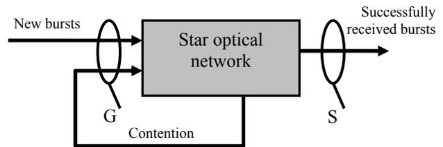
**Fig. 1** A star optical network with retransmission scheme
