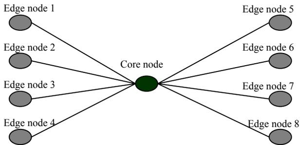
**Fig. 2** Star topology with 8 edge nodes
