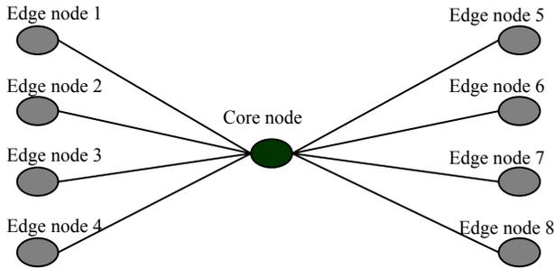
**Fig. 2** Star topology with 8 edge nodes
