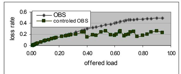
**Graph 2.** Loss rate as function of load with and without congestion control
