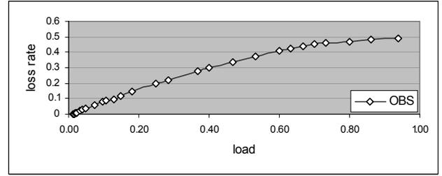
**Graph1.** Loss rate as function of load
